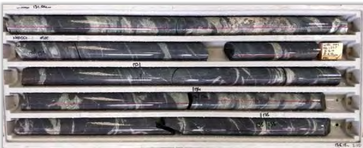
Core from 20WHD001, 131-135.15m (sphalerite at 131.6m)
