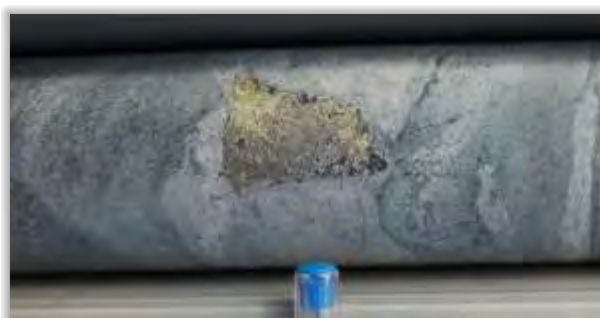
Clast of pyrrhotite - pyrite - ?chalcopyrite (125.6m)
