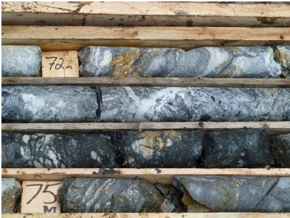
Figure : Section of Type 2 mineralisation - brecciated, sulphide-bearing (including some sphalerite) quartz-carbonate-graphite stratabound metasedimentary unit, up to 20m thick (DDH 3).
