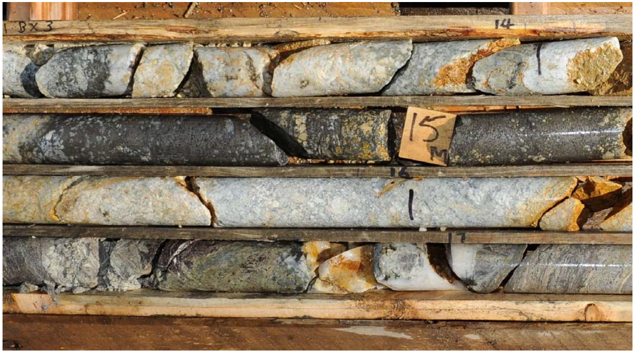
Figure : Section of about 0.5m of semi-massive sulphide, pyrrhotite-pyrite-sphalerite, from DDH 4 (trench area) at 15m depth – Type 1 mineralisation
