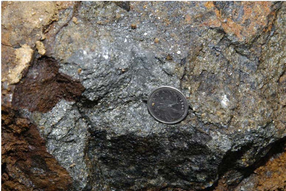
Trench 1 – Massive pyrite-pyrrhotite sample with anomalous molybdenum and rhenium. Part of a 400m long magnetic anomaly with a coincident, discrete EM anomaly detected by helicopter borne EM survey, October 2011.
