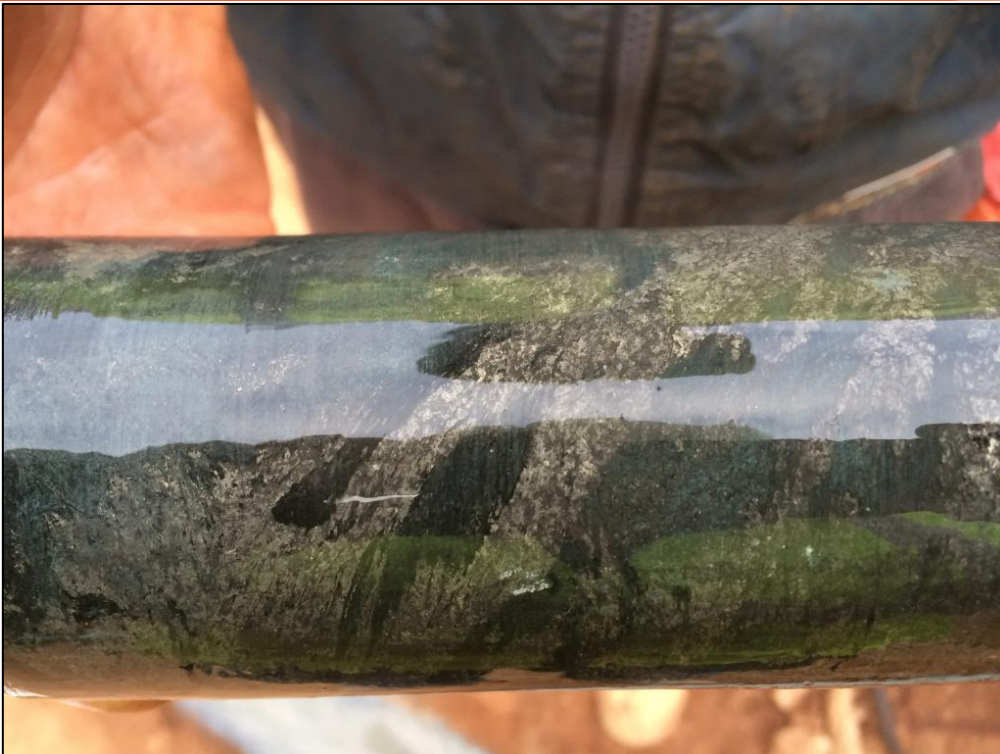
Figure 2: Semi Massive pyrrhotite pentlandite (XRF to 3.15% Ni), KLDH01 93.15 - 93.35m
