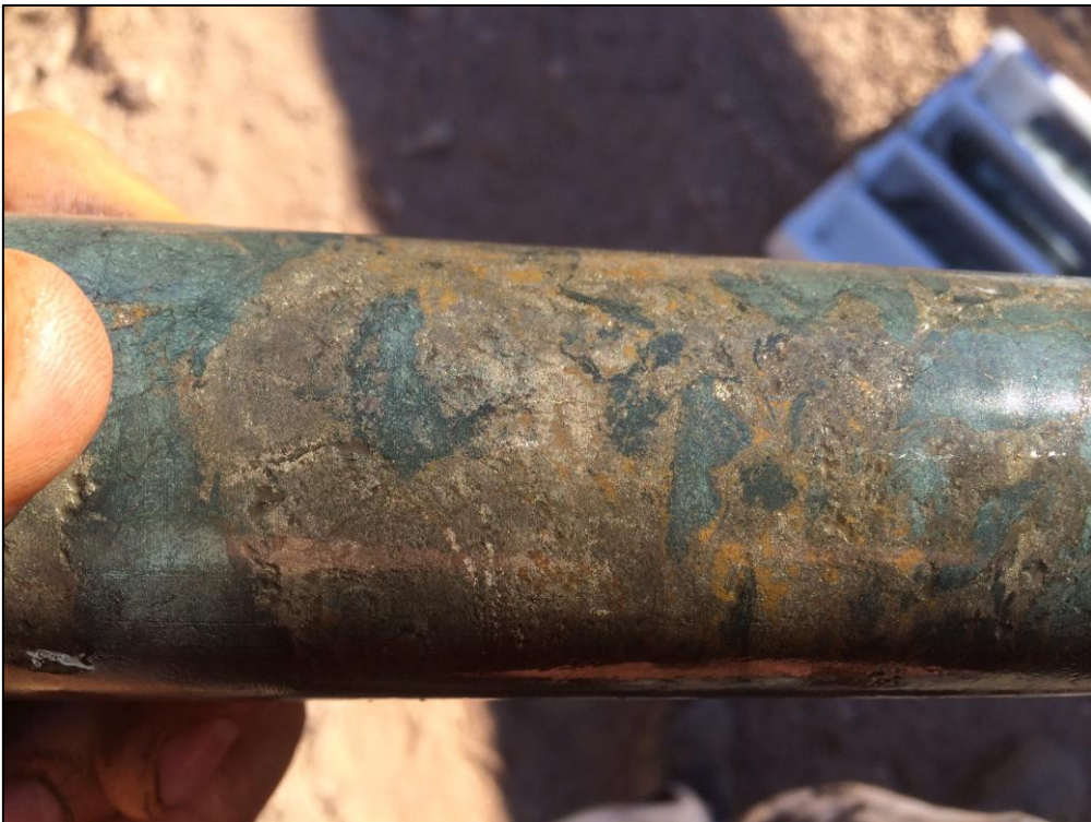
Figure 3: Semi Massive pyrrhotite pentlandite (XRF to 1.75% Ni), KLDH01 137.5 - 137.7m
